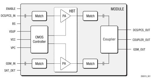
Figure 1. SKY77331 Functional Block Diagram
